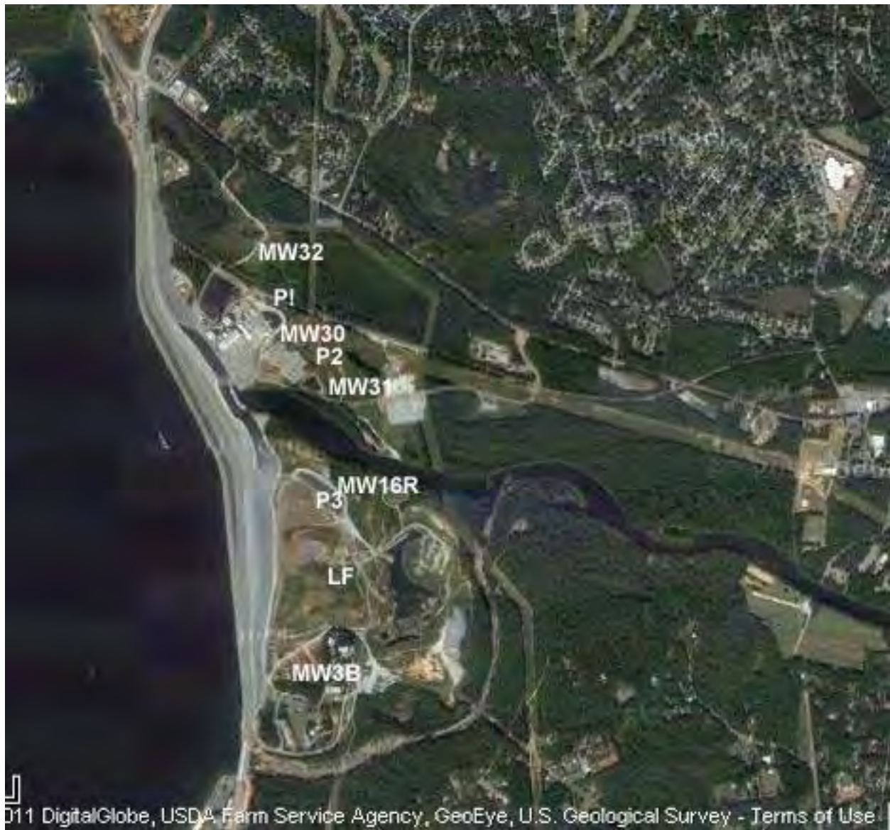
McMeekin Station Active Landfill (LF), Pond P1 (Coal Pile Runoff), Pond P2 (Low Volume Waste), Pond P3 (Wastewater), and Monitoring Well Locations.
