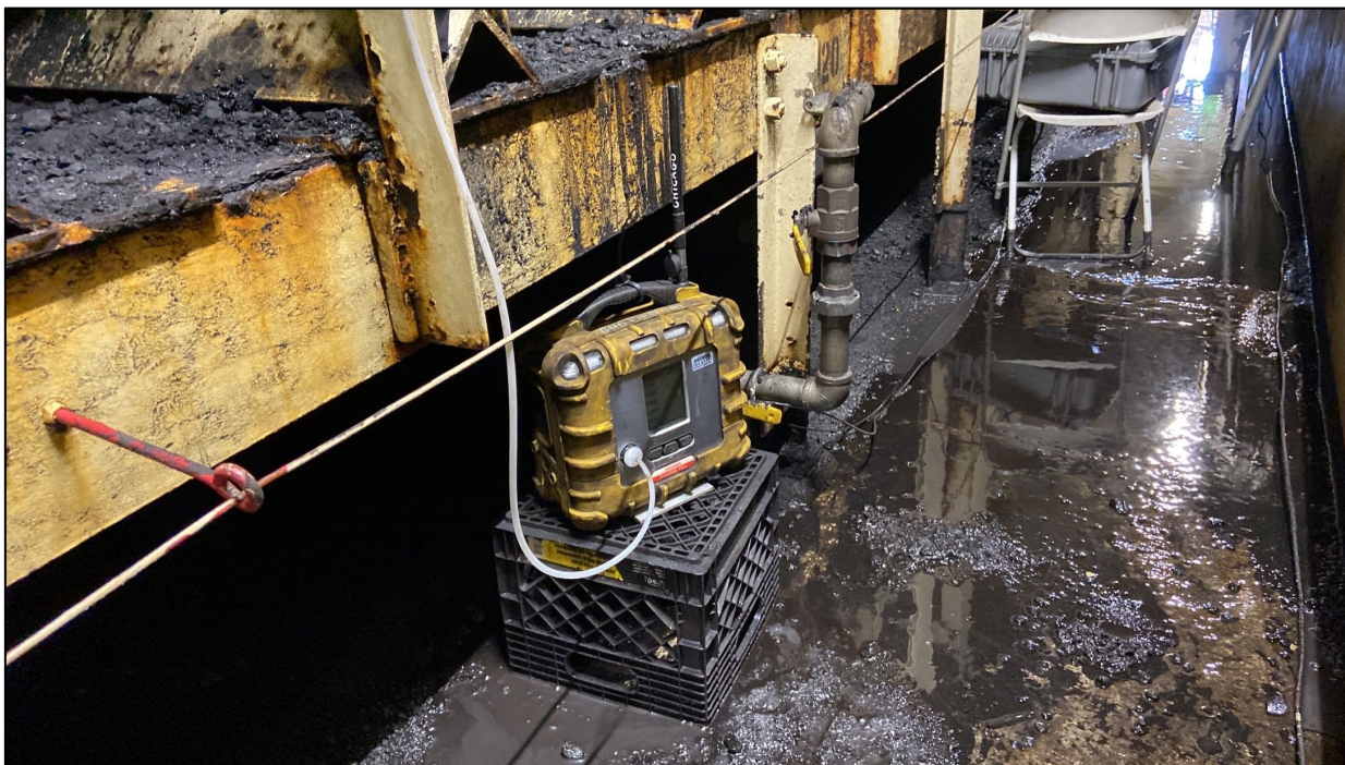
Figure 5.6.2. Monitoring high location near top of tunnel using tubing.
