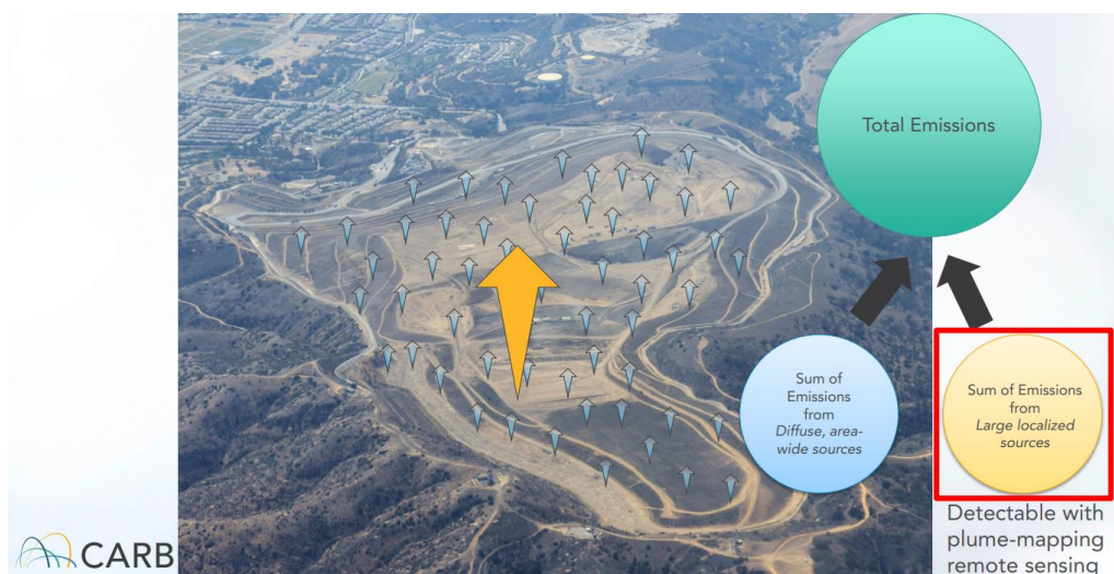
Figure 1: California Air Resources Board graphic showing that landfill emissions can include large plumes and smaller diffuse emissions spread over the surface of the landfill. 21
