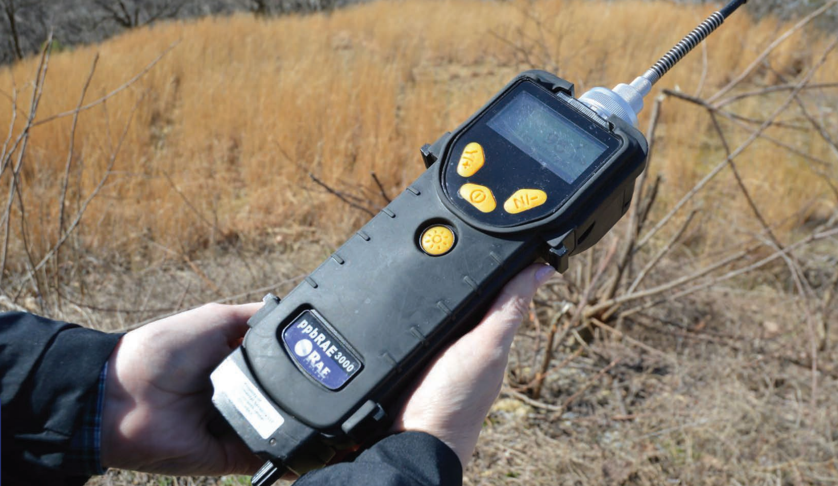
Air monitor used by local volunteers to measure emissions from the Shell Monaca plastics plant in Pennsylvania.
