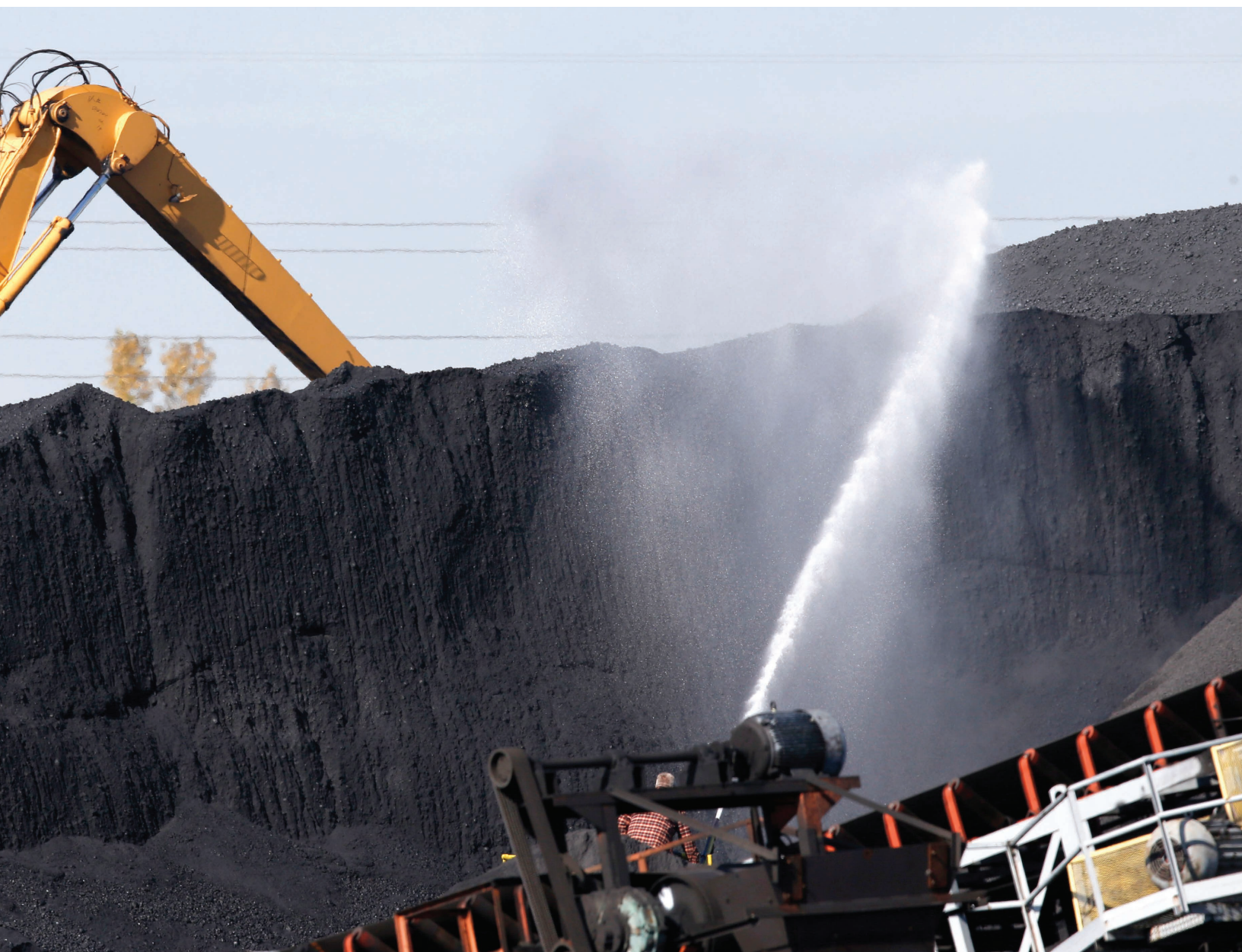
A pile of petroleum coke is watered down to prevent dust from blowing into the nearby community. It was located at a petcoke transfer facility along the Calumet River on Chicago's southeast side.
