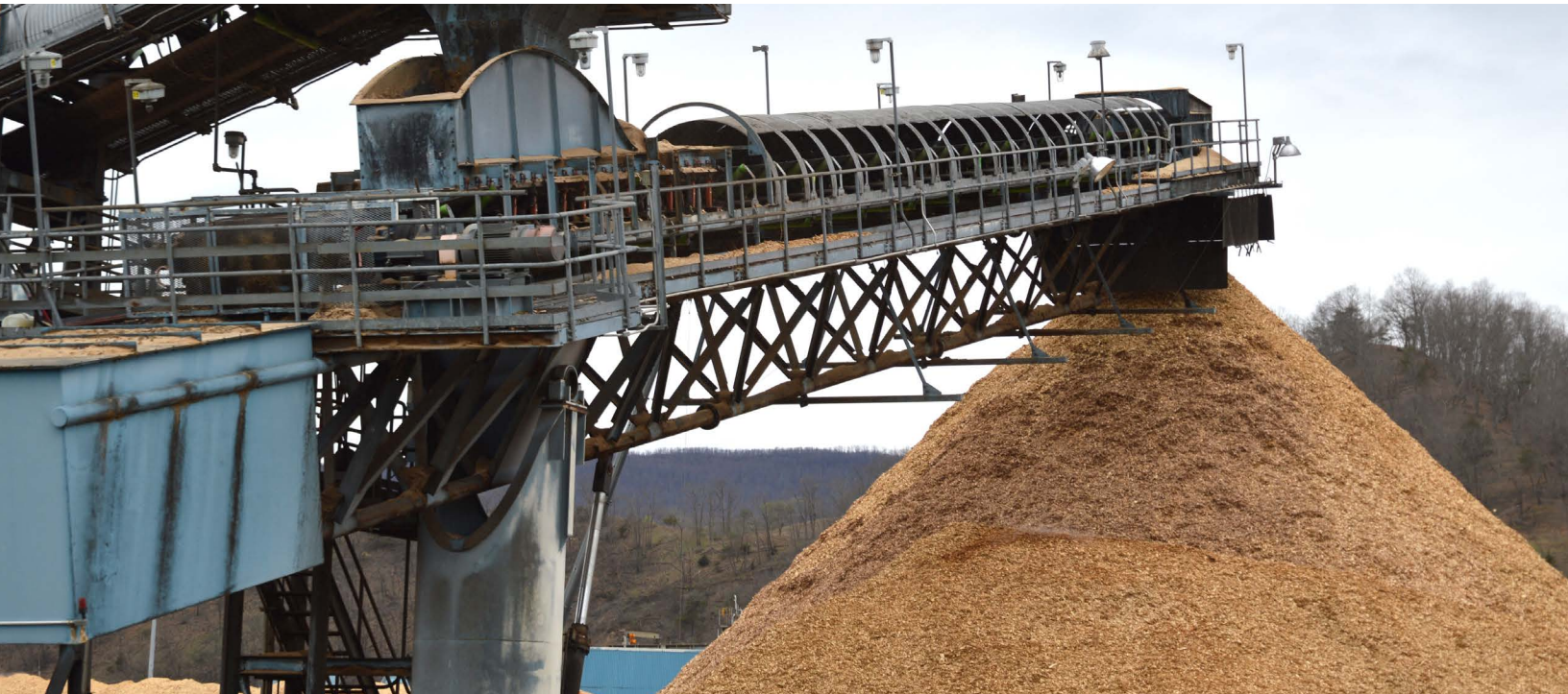
Trees are chipped as the first step of making pulp in the paper manufacturing process. Paper mills with outdated equipment release large amounts of pollution into local communities, including hydrogen sulfide, particulate matter and sawdust.
